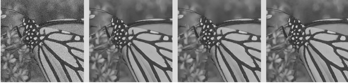
Figure 6. Denoising performance comparison for monarch image: a) noisy ( \sigma_w = 20 ); b) BM3D ( PSNR = 30.37dB , SSIM = 0.9209 ); c) K-SVD ( PSNR = 29.89dB , SSIM = 0.9075 ); d) CSR ( PSNR = 30.70dB , SSIM = 0.9197 ).
